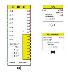
Developed digital twin of the fail-safe modules: (a) Fail-safe digital input with 8 inputs. The yellow box in the components marks the value status bits – bits that signal errors in the given channel. (b) Fail-safe digital output module that shows maximum reaction time and (c) block that summarizes all maximum reaction times.
